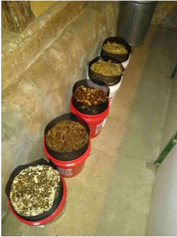
Figure 2. Carbon amendments evaluated in repetition 1, prior to slurry application. Shown are (top to bottom) are CS, ConCS, SD-PWC, Mulch, SD-LFS.
