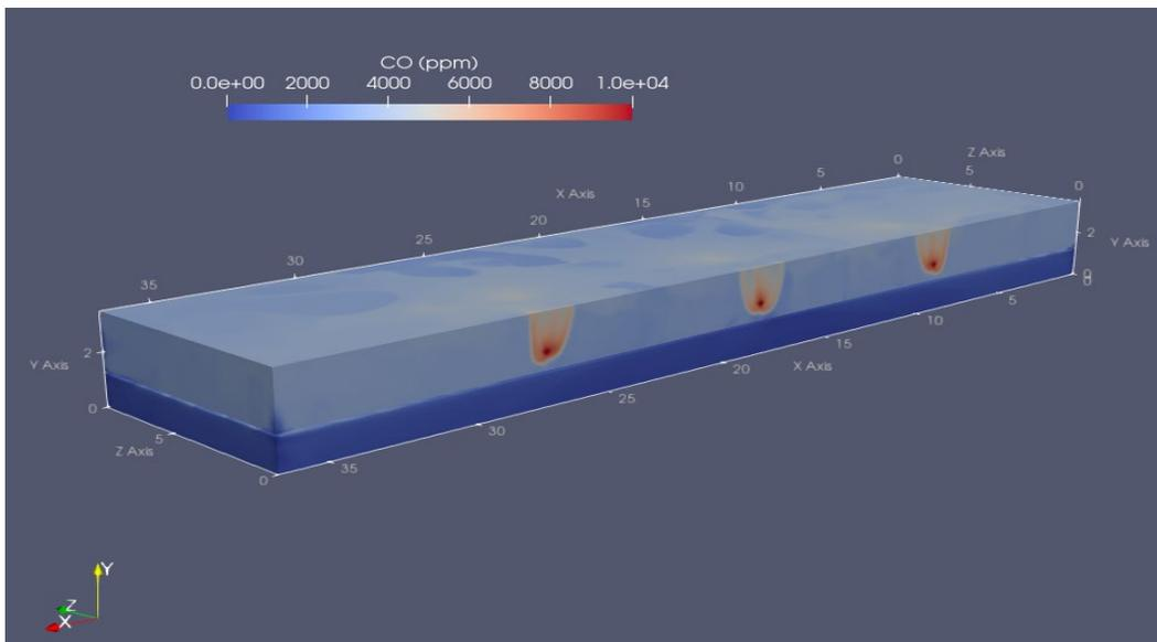
**Figure 8: Time snapshot at t = 1800 s of the CO concentration in the barn (exterior view), with inlet visible. Coordinates are in meters (1 m = 3.2808 ft). Simulation with 1.5 ACH and heat source due to the animals.**
