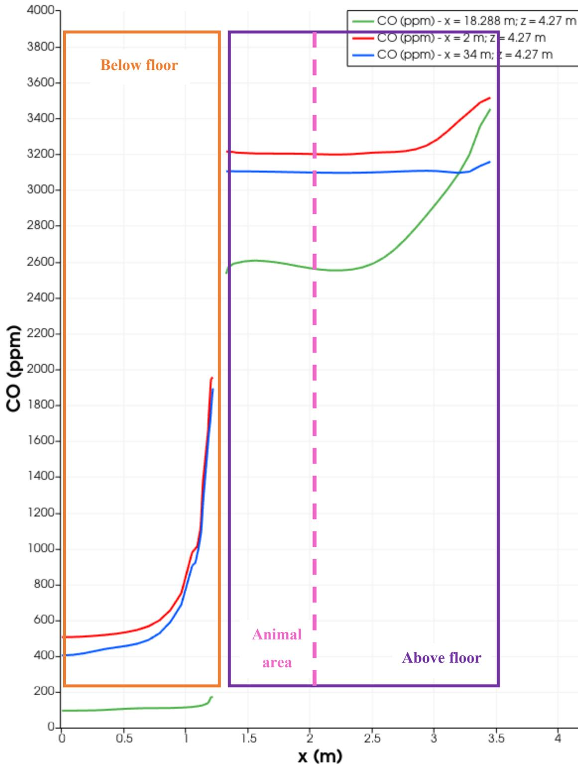
Figure 11: CO concentration at  $t = 1,800$  s along three vertical lines spanning the entire height of the barn. Simulation with 1.5 ACH and heat source due to the animals.
