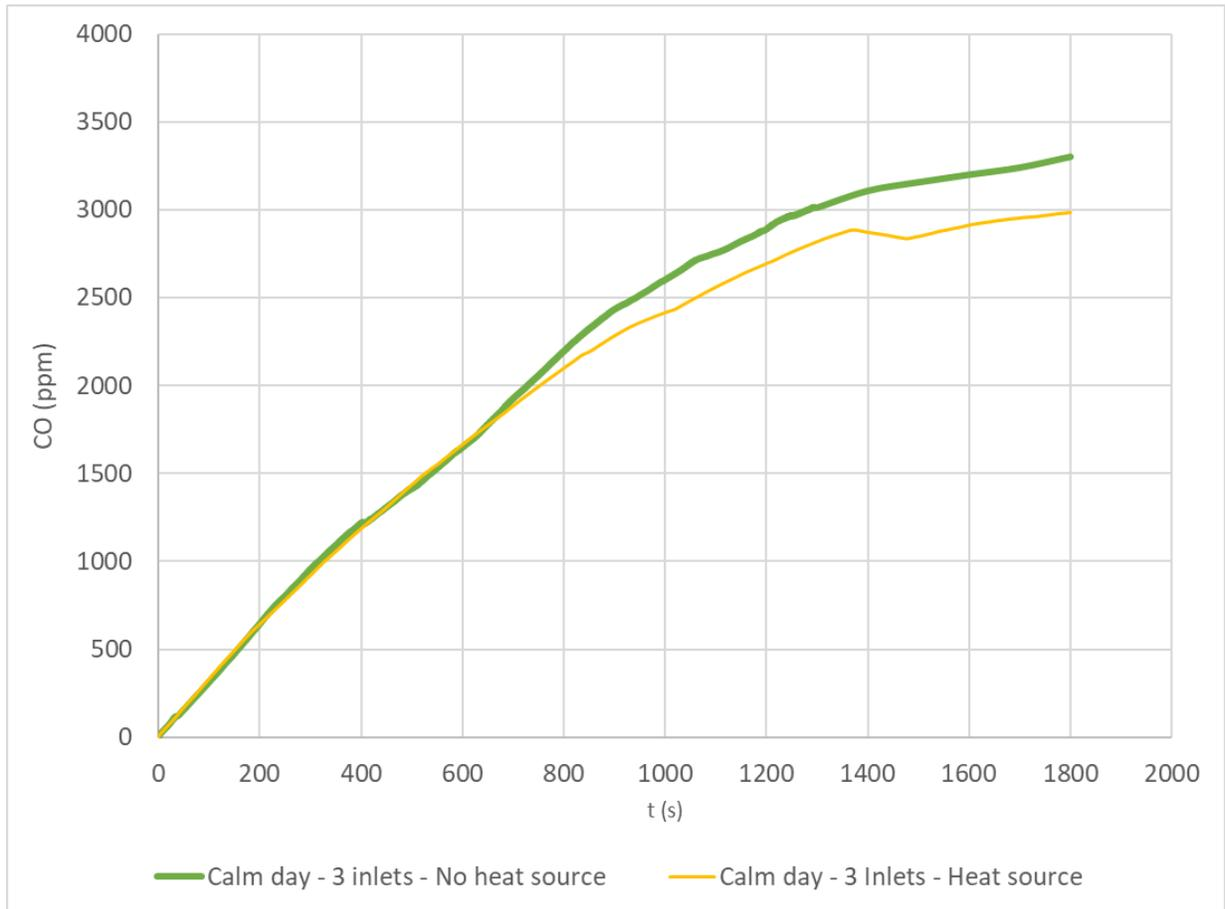
**Figure 7: Time evolution of CO concentration in the upper part of the barn with three inlets. A calm day was assumed to correspond to 1.5 ACH.**
