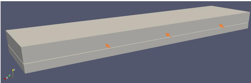
Figure 4: Schematic of the barn in the CFD simulations and location of the three inlets.
