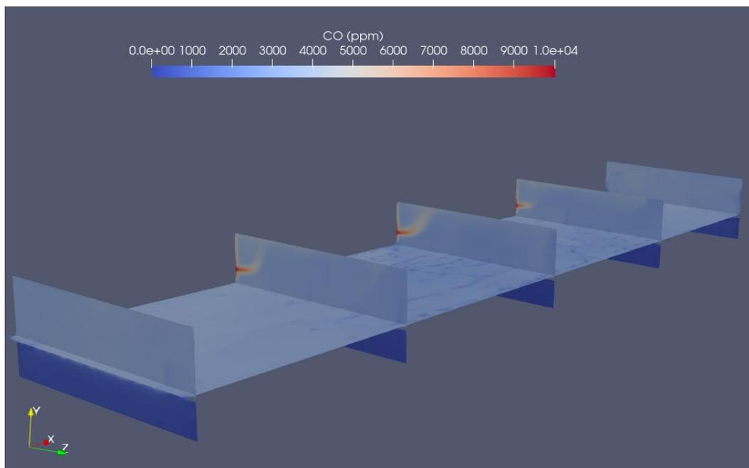
**Figure 10: Contour of CO concentration in the barn at  $t = 1800 \text{ s}$  over several vertical planes. The horizontal plane is at floor level. Simulation with 1.5 ACH and heat source due to the animals.**
