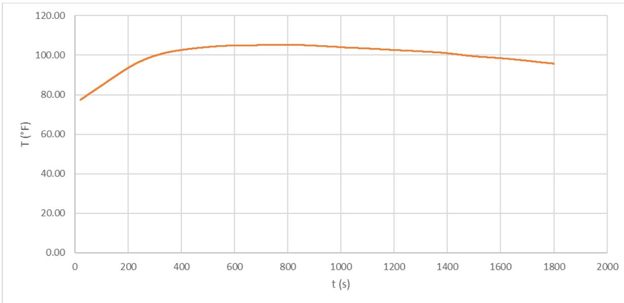
**Figure 9: Average temperature inside the barn with three CO injections and heat source.**
