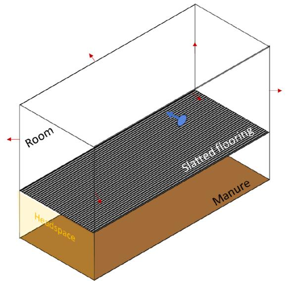
**Figure 1: Schematic representation of the barn.**
