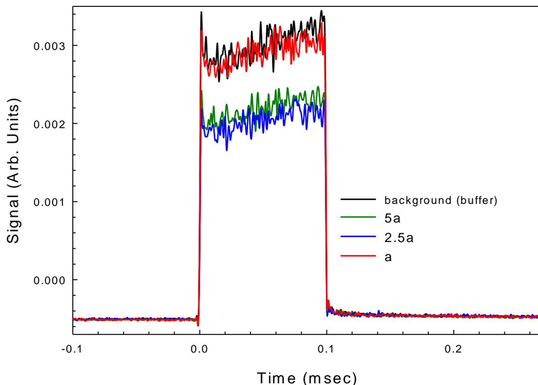
Fig. 7. Actual photoluminescence signals produced by the OLED excitation using different concentrations of R-IgG antibodies; *a*, *2.5a*, and *5a*, antibody concentrations of 1X, 2.5X and 5X, respectively.
