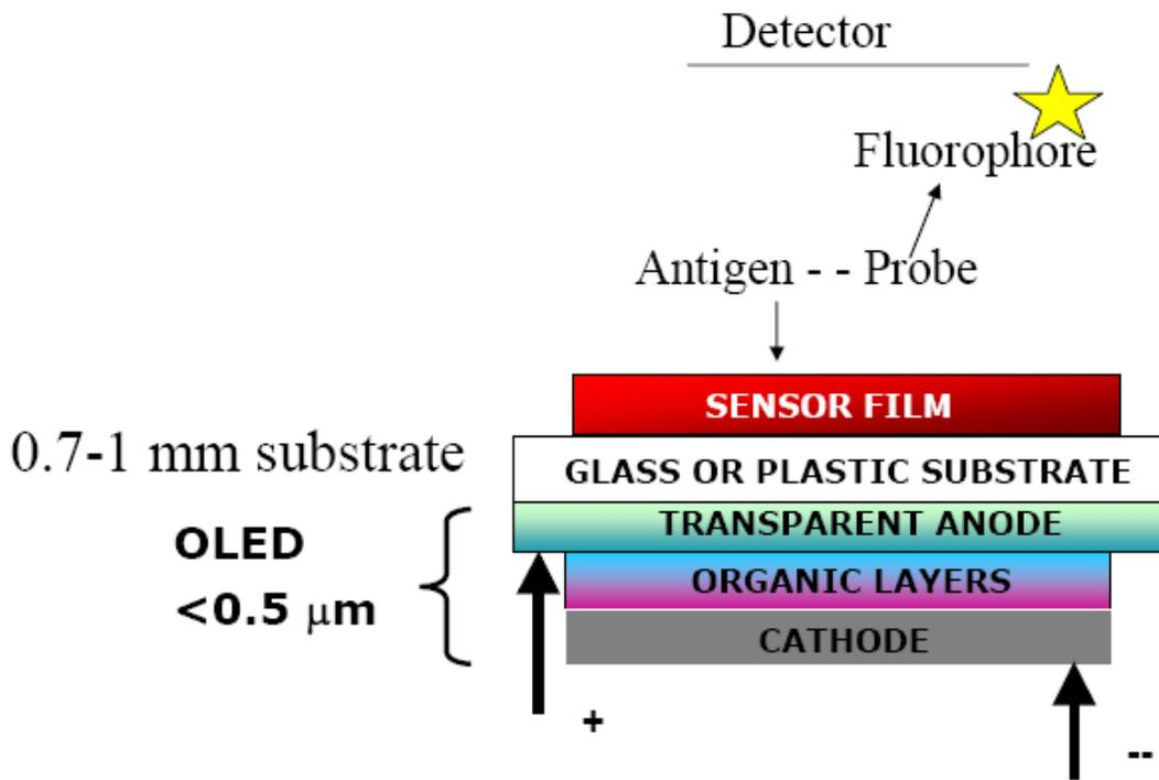
Fig.8 Schematic of an OLED detection system.
